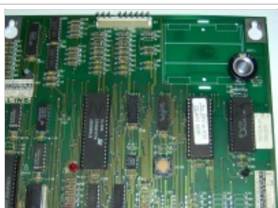
Installation of a Memory Capacitor
