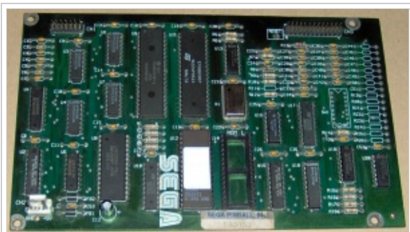
Sega White Star Display Controller Board
