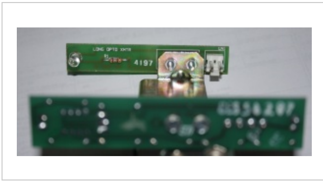
The opto transmitter side.
