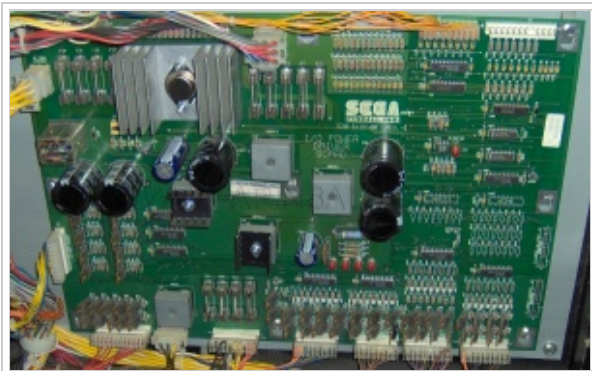
Stern White Star I/O Power Driver Board
