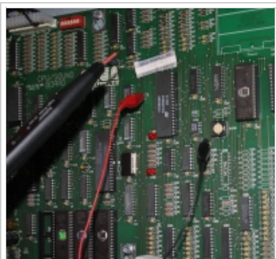
Connecting a logic probe to a Sega/Stern White Star MPU
