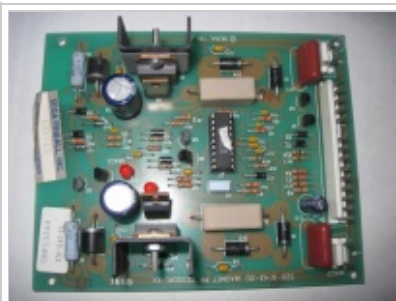
Sega 520-5143-00 Magnet Processor Board
