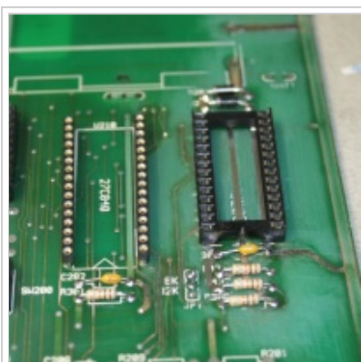
Bare copper traces tinned.
