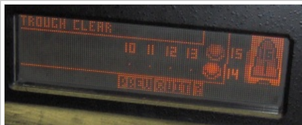
A Stern Monopoly in "Clear Ball Trough" Mode Identifying One Ball in the Trough and One Ball Stacked
