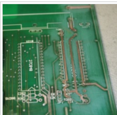
More components removed, the alkaline damaged traces sanded, and the damaged area treated with 50/50 vinegar and water.
