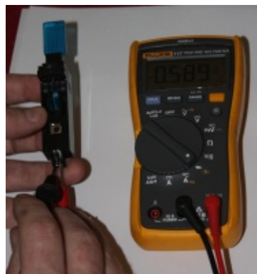
Testing a closed target switch, step 2. In diode test, with the switch closed, your meter should read .5 to .7, the nominal voltage drop across a diode.
