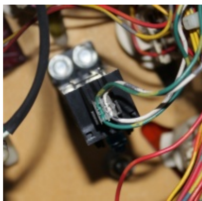
The Achilles Heel of a Sega target...the IDC connector.
