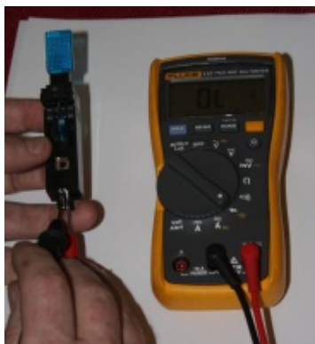
Testing a closed target switch, step 1. In diode test, with the switch closed, your meter should read 0 or null.
