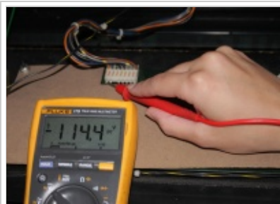
Testing DMD Controller voltages at the display. Note: This picture is a Williams game, but the concept is the same.
