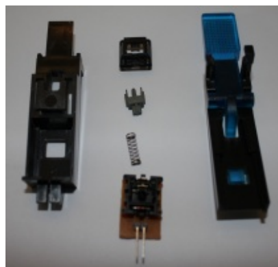
"Exploded" target parts. The gray switch part must be oriented correctly. Note the integrated diode just under the micro-switch, center/bottom.
