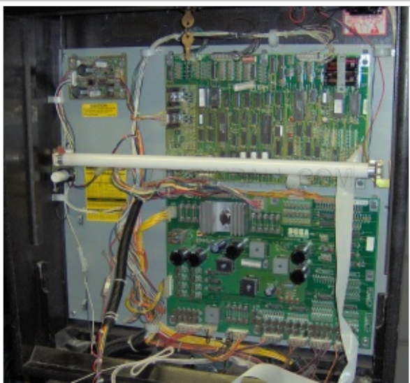
Typical Early Stern White Star Boardset (Monopoly)
