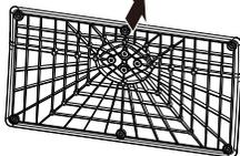
**3** Fix the base stand to the TV using the 4 pcs provided screws.
