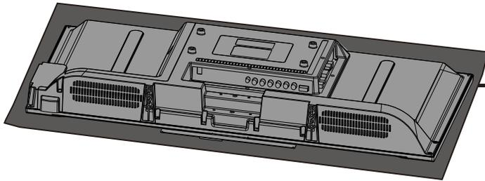
**1** Lay the TV face-down on a flat, cushioned surface to avoid the screen from damage or scratches.
