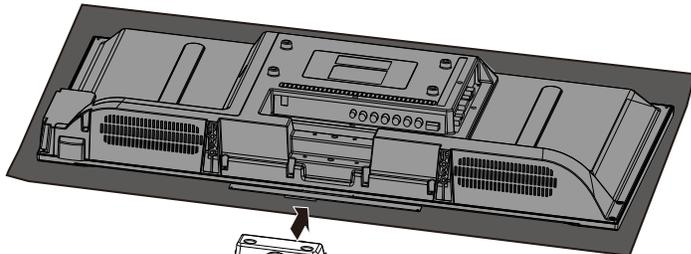
**2** Fix the stand support to the TV using the 4 pcs screws.
